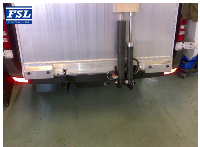
Housings manufactured to include original Mercedes Benz parking sensors.
